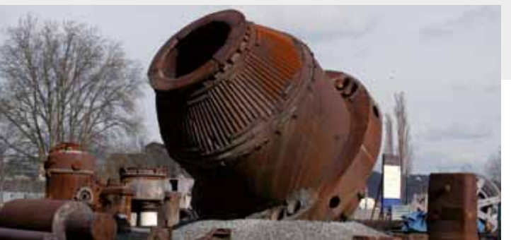
The steel converter
